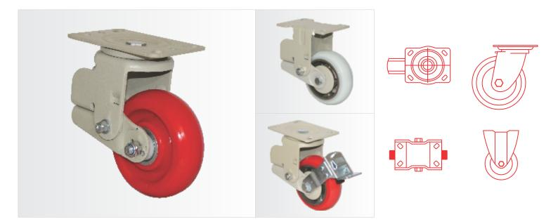
Heavy Pressed Steel Spring –Loaded Castors to absorb the shocks/ vibrations during loadings with controlled impact. Top plate & bracket of our Castors are made out of thick sheets to provide strength & ensure that the load is evenly distributed over wheel & spring assembly.
