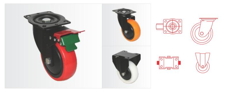
Medium Duty Pressed Steel Castors having double ball bearing in Swivel head with thick threaded King Pin to avoid dust. Fitting available in Plate, Stem (Round/ Square) in Chrome Plated/Powder Coated /Zinc Plating.
